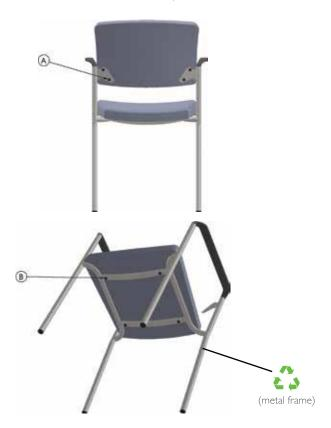
A & B: Using a #2 Philips screwdriver remove the back (four screws) and the seat (four screws). Two 5/32" Allen keys are required for those with exposed wood backs.
