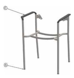
**C:** Place the chair frame upside down. Using pliers firmly secure and twist the four glides free from the legs.
